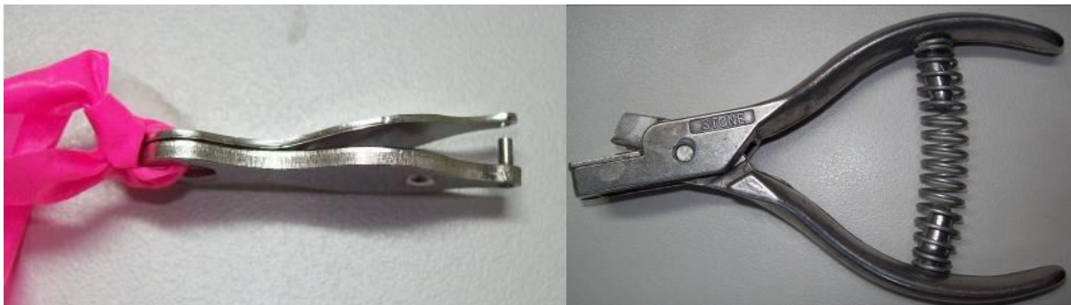
Figure 1 A 2mm ear punch (left) and ear notcher (right). Flagging tape is attached to the ear punch to increase visibility to prevent it from being easily lost. Photo: Vanessa Richter/DBCA.
