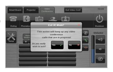
**NOTE:** Letting the system go to sleep by itself only powers down the touch panel screen, it **does not turn off** the audio-visual equipment. To turn off the equipment, shutdown the system properly using the touch screen panel. This will extend the life of the audio-visual equipment.
